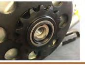
Install the grease trap with the sprocket side facing the sprocket. The sprocket side is stamped "SPROCKET SIDE".
