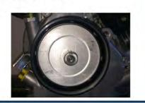
Install a 3/4" x 1 1/16" O.D. x .04" thick steel washer against the crankshaft spacer.
