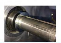
STEP 9 Install the 34" x 2 14" O.D. x 1/16" thick spring/shoe retaining washer.
